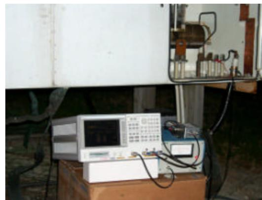
IMPEDANCE MEASUREMENTS AT ATU INPUT
